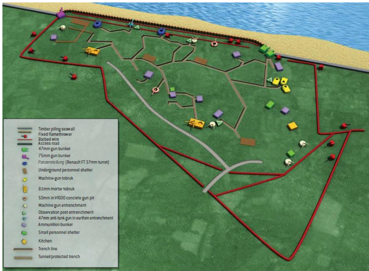
ABOVE: Strongpoint WN10, Les Dunes de Varreville. WN10 was a fairly typical infantry resistance nest containing a mixture of reinforced concrete bunkers and earthen entrenchments. This was one of three inter-related strongpoints manned by 4. Kompanie, Infanterie-Regiment 919, 709. Infanterie-Division, and located to the north-west of Utah Beach, covering an area 600m wide and 300m deep. (Chris Taylor @ Osprey Publishing)
