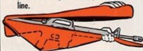
2. If absolutely necessary, you can fire right through the bag. You can operate the selector lever and trigger easy with the bag on. But, remember this: Ejected cases will be trapped in the bag and could cause a malfunction after the first round. So get it off as quick as you can.
