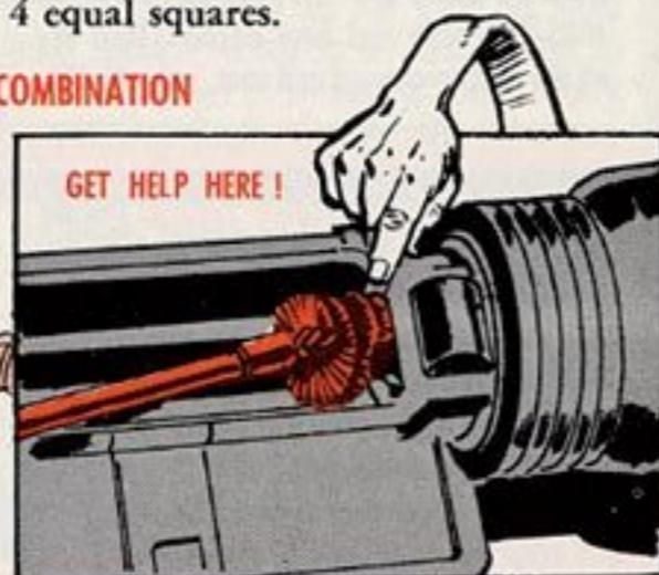
with crud or carbon buildup when you're cleaning your rifle—especially in the bolt and locking recess area—get your armorer to help you tackle it with P-C-111 carbon removing compound, FSN 6850-965-2332, 5-gal pail.
