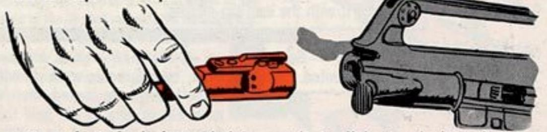
Here's the Pitch: The front end of the gas tube is self-cleaning, thanks to the hot gases and high pressure from the barrel. But, if you don't keep the other end clean—the gas tube area where it mates with the carrier key inside the receiver—brother! You've got to clean this area with elbow grease to prevent stoppages. Hear!
