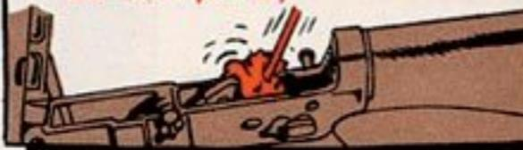
3. Wrap a piece of clean cloth or cleaning patch around the brush handle and poke it into the hard-to-get-at places. Do the best job you can to get rid of carbon and gunk that could keep the parts from working right.
