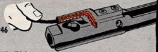
3. Use another pipe cleaner—or air-dry it by waving it around—to dry the tube as well as you can.
