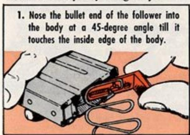
1. Nose the bullet end of the follower into the body at a 45-degree angle till it touches the inside edge of the body.
