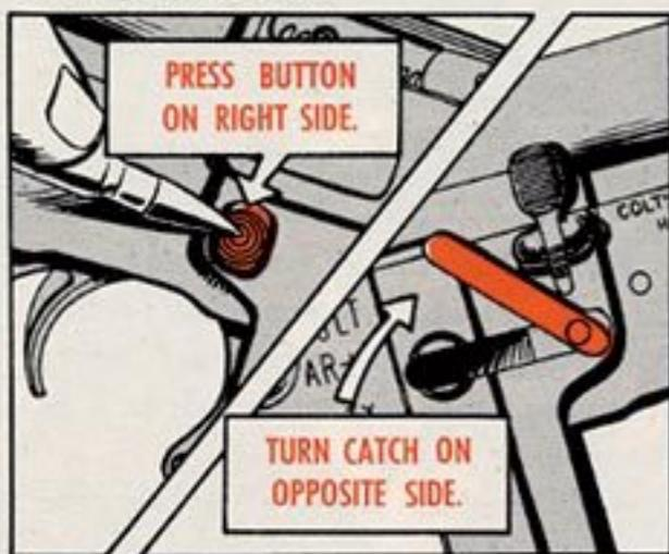
No sweat adjusting the catch the way you want it, either . . . and you're authorized to pull this deal. Just press the button on the right side of the rifle with the nose of a cartridge far enough so's you can turn the catch on the left side of the weapon. You turn the handle clockwise to tighten it and counter-clockwise to loosen it. Best of all, you don't have to take the weapon apart to do this.
