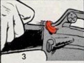
If a cartridge or case is ejected, release the charging handle to feed a new round.
