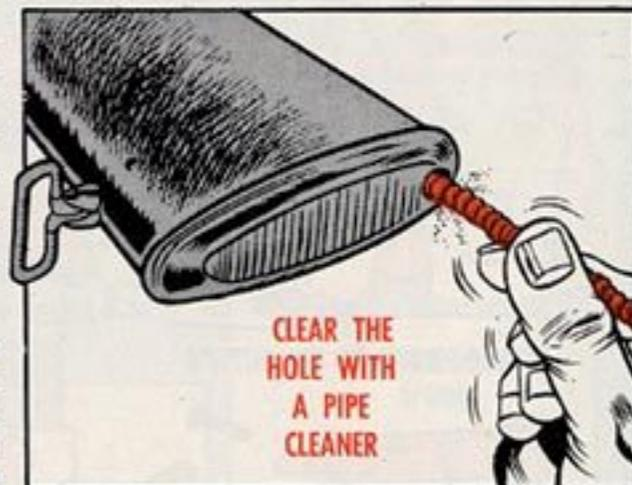
it'll foul up the working parts . . . cause corrosion and dampen your ammo.
