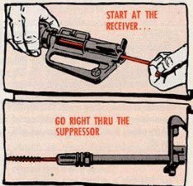
Same idea goes when you're running patches through. Run it all the way through the flash suppressor before you start to pull back . . . no matter what size patches you're using—the one for the M16A1 (FSN 1005-912-4248) or any large type that you have to cut into 4 equal squares.
