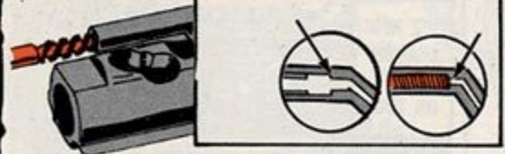
Make sure you get the metal end of the brush in all the way—right into the bottom of the hole where the gas tube is seated in the carrier key—and then turn it to loosen the crud. That last 1/16-in in there is the most neglected part on most M16A1 rifles.
