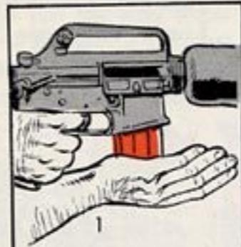
Tap upward on the magazine to make sure it's seated right.
