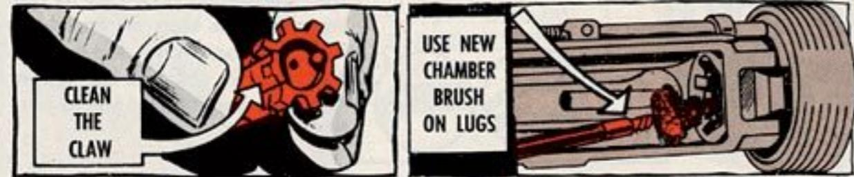
collect under the extractor, the claw won't be able to snap over the rim of a cartridge case. And if gook and brass chips from cases gather in the recesses, your bolt action will be stymied. So, bear down on your bore brush in both these places.
