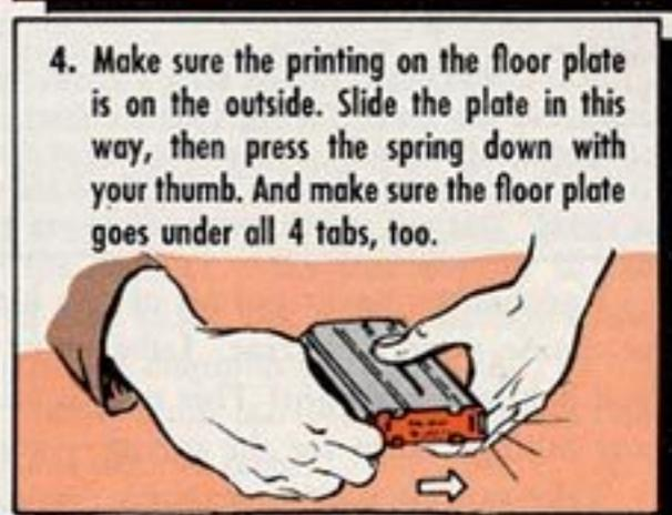
4. Make sure the printing on the floor plate is on the outside. Slide the plate in this way, then press the spring down with your thumb. And make sure the floor plate goes under all 4 tabs, too.
